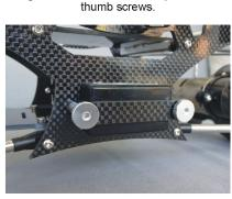
Velcro straps can be fed through the slots under the battery tray without removal.
