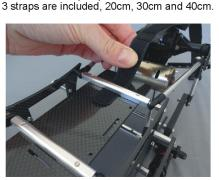
The 40cm can run the length of the battery tray to hold a regular length 2s pack.
