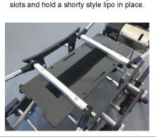
It is possible to install the battery with the top deck in place, it has been removed here to show the layout.
