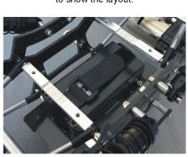
The 20cm strap can be used through the side slots as extra security to hold the battery pack in place.
